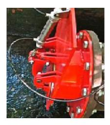
The CheckValve<sup>™</sup> is a pneumatically activated unit which contains pollutants, oil spills and firewater run off issues on site within seconds of an incident.
